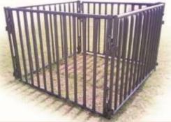
All hog & sheep components are constructed from A-513 high tensile steel tubing. All joints are saddle cut for extra strength. Gate frame is 72" tall and panels are available in 41" or 48" height. All units interlock with self contained drop pins. All components are finished with a long lasting powder coat finish.
